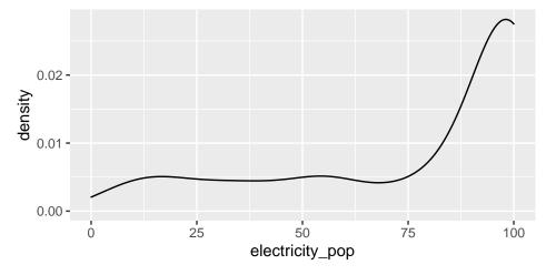
If you do not want the density graph to be plotted as a closed polygon, you can instead use the <code>geom\_line()</code> geometric object function with the <code>stat = "density"</code> parameter.
